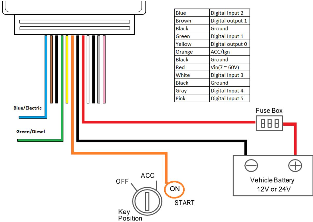
All digital inputs of the TLW2-12BL supports voltage of up to 60V.
